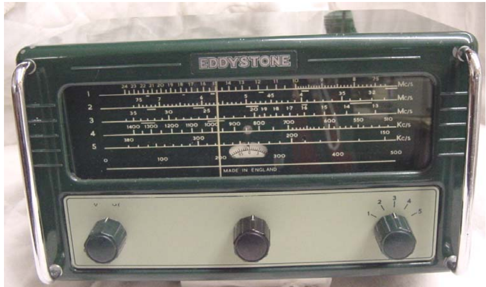
The S.870A's simple control panel – note the five wavebands and the 'reverse' tuning
