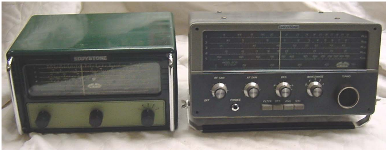
Above An S.870A next to a (slightly worse-for-wear and modded/bits missing) EC10 MkI - note that the S.870A is significantly smaller than its younger and solid state sibling
