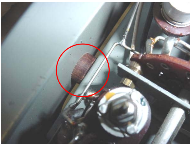
Above left: Paxolin insulating washer between the chassis and inner case sides; Above right: Band change switch shaft isolated from front panel
